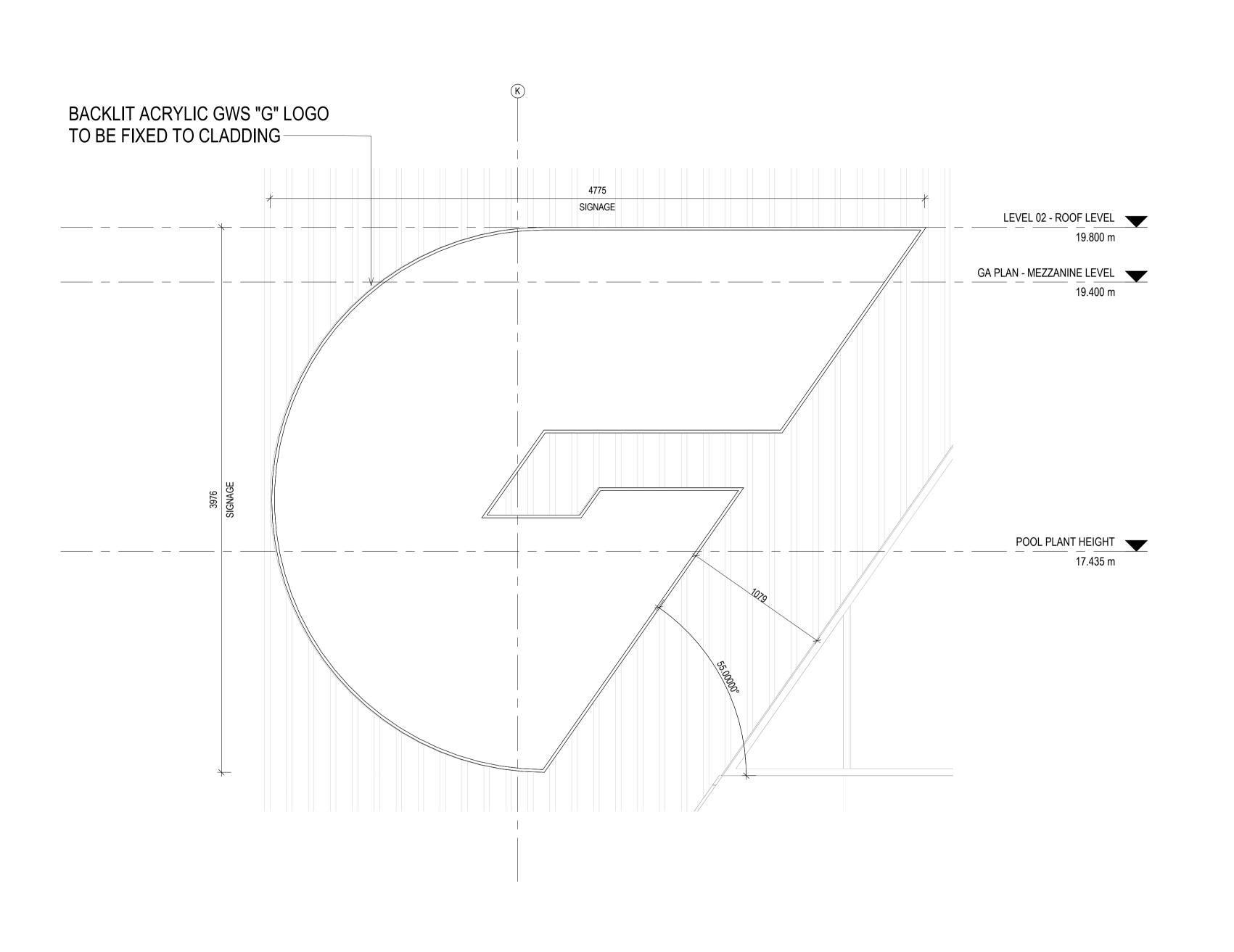
REFERENCE MAP FDC LANDSCAPE ARCHITECT COST CONSULTANT DISCLAIMER USE FIGURED DIMENSIONS ONLY DO NOT SCALE FROM DRAWING CHECK & VERIFY ALL DIMENSIONS ON SITE BEFORE FABRICATION OR SET OUT. This drawing is diagrammatic and shows general arrangements.
